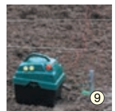
9 Attach and earth the energiser
