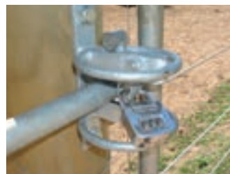
Advantage 3: lockable, padlock (optional extra)
